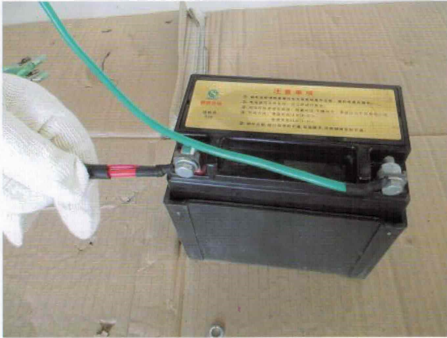
Step 25. Close the cap of the battery box, place the red wire and green wire at the gap of the seal.
